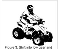
Figure 3. Shift into low gear and point the ATV directly downhill when descending a slope
