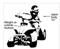
Figure 1. Turning. Lean your upper body toward the inside of the turn while keeping your weight on the outer footrest
