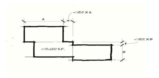
This diagram is an example of how separate Building Elements could maintain compliance with the square foot maximum called for, while being part of a larger structure. The block below and to the right of the uppermost block is attached to a wall the length of A and is offset by 15% of
